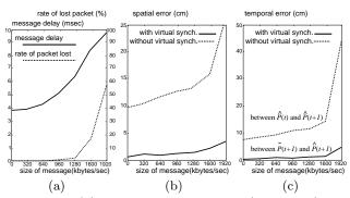
Figure 13: (a) Delay of the message (solid line) and Rate of lost packet (dotted line), (b) Error in spatial object identification, (c) Error in temporal object identification.
